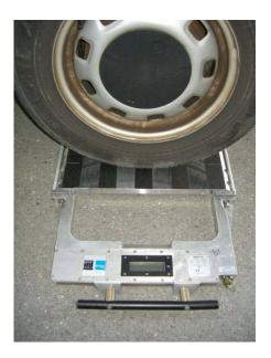
Figure 6 - Tyre position on scale
