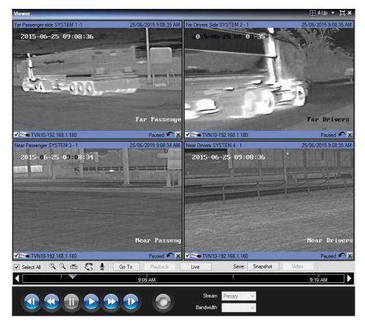
The configuration of the cameras allowed for the footage to be viewed in order of Camera number with a slight delay between images. This allowed the user to view both sides of the whole vehicle and decide whether to advise the RMS operator to manually bring the vehicle in for a secondary examination.
